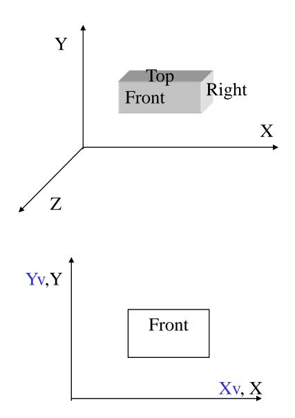
Geometric Transformations for Generating Orthographic Projection (Front View)
