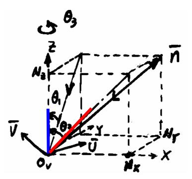
Then, rotate  $\theta_3$  about the Z axis to align  $\bar{u}$  with X and  $\bar{v}$  with Y
