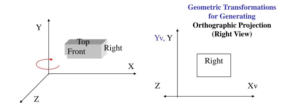
$$P_{\nu} = \begin{bmatrix} 1 \ 0 \ 0 \ 0 \\ 0 \ 1 \ 0 \ 0 \\ 0 \ 0 \ 0 \ 0 \\ 0 \ 0 \ 0 \ 1 \end{bmatrix} \begin{bmatrix} \cos(-90^{\circ}) & 0 & \sin(-90^{\circ}) & 0 \\ 0 & 1 & 0 & 0 \\ -\sin(-90^{\circ}) & 0 & \cos(-90^{\circ}) & 0 \\ 0 & 0 & 0 & 1 \end{bmatrix} P = \begin{bmatrix} 0 \ 0 \ -1 \ 0 \\ 0 \ 1 & 0 & 0 \\ 0 \ 0 & 0 & 0 \\ 0 \ 0 & 0 & 1 \end{bmatrix} P$$
