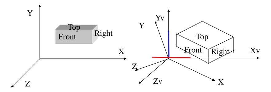
$$P_{v} = [R]_{x}^{\phi}[R]_{y}^{\theta}P = \begin{bmatrix} 1 & 0 & 0 & 0 \\ 0 \cos \phi & -\sin \phi & 0 \\ 0 \sin \phi & \cos \phi & 0 \\ 0 & 0 & 0 & 1 \end{bmatrix} \begin{bmatrix} \cos \theta & 0 \sin \theta & 0 \\ 0 & 1 & 0 & 0 \\ -\sin \theta & 0 \cos \theta & 0 \\ 0 & 0 & 0 & 1 \end{bmatrix} P$$
