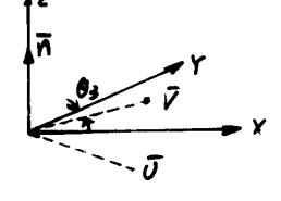
We need to rotate by an angle  $\theta_3$  about the Z axis
