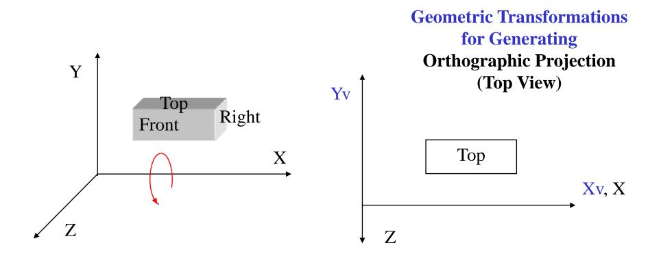
$$P_{v} = \begin{bmatrix} 1 & 0 & 0 & 0 \\ 0 & 1 & 0 & 0 \\ 0 & 0 & 0 & 0 \\ 0 & 0 & 0 & 1 \end{bmatrix} \begin{bmatrix} 1 & 0 & 0 & 0 \\ 0 & \cos(90^{\circ}) & -\sin(90^{\circ}) & 0 \\ 0 & \sin(90^{\circ}) & \cos(90^{\circ}) & 0 \\ 0 & 0 & 0 & 1 \end{bmatrix} P = \begin{bmatrix} 1 & 0 & 0 & 0 \\ 0 & 0 & -1 & 0 \\ 0 & 0 & 0 & 0 \\ 0 & 0 & 0 & 1 \end{bmatrix} P$$
