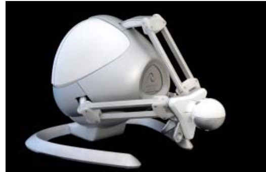
Figure 3. The NOVINT FALCON 3 DOF haptic device.
