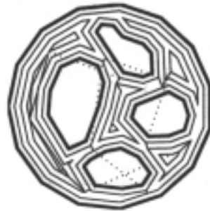
(b) Stock-offset tool path pattern
