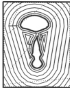
(b) Stock-offset tool path pattern
