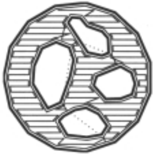
(a) Parallel tool path pattern
