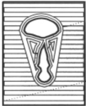
(a) Parallel tool path pattern
