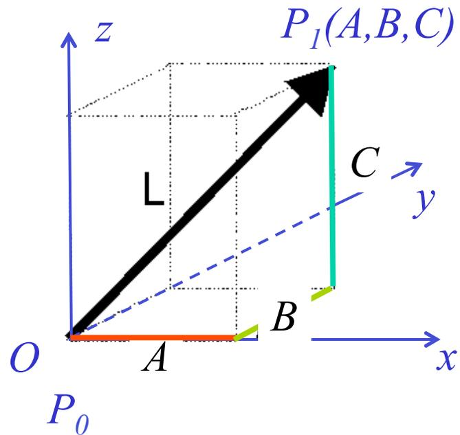
Step 2: Rotate Vector about X Axis to get into the x - z plane
