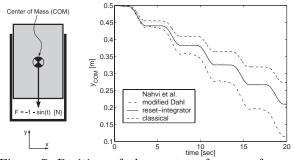
Figure 7: Position of the center of mass of a peg pushed in a hole with friction (simulation).
