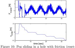
Figure 10: Peg sliding in a hole with friction (resetintegrator).
