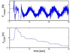
Figure 9: Peg sliding in a hole with friction (driftless Dahl [10]).
