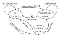
Figure 3: The contact states of one collision pair.
