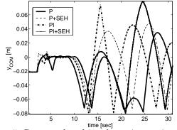
Figure 5: Rectangular object bouncing against marginally passive and active walls (experiment).
