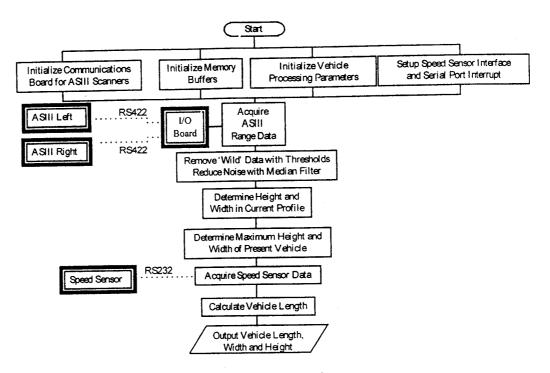
Figure 2 Functional Modules of the AVDMS
