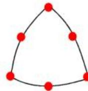
Parabolic triangular element
