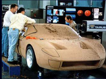
Scanning of Clay Model to Obtain Surface Data
