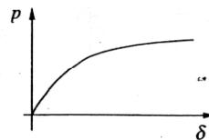
This is a geometrically nonlinear (large deformation) problem and iteration method (incremental approach) needs to be employed.
