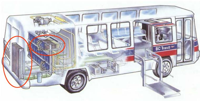
One of the key design challenge - getting rid of the low grid heat using an inefficient stainless radiator
