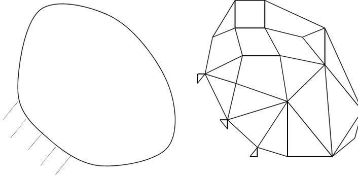
Task of FEA: To identify and solve the stiffness equations for a system of “finite elements.”
