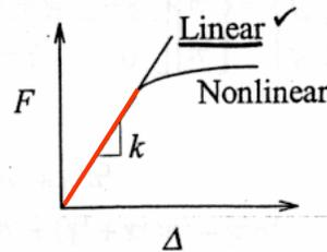
$k = F / \Delta$  ( $> 0$ ) is the force needed to produce a unit stretch.
