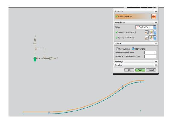
For creating the edge of the part, a different set of steps is required. The functionality of the move objects tool set seems to be limited in that it will not allow copying of entities from one sketch into another. To overcome this, model geometry will be converted instead.
