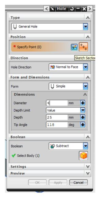
> Selection Criteria may be narrowed by the Hole Direction pull down menu. An existing reference or geometric point may be selected under Position, or the position may be defined by generating a sketch. **click** on the SKETCH SECTION button.
