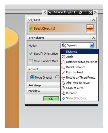
Here we choose an entity to transform. Transformations allow either moving an object, or copying an object with the new locations parameters. We can:
